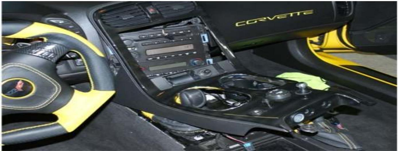
The Picture below is the EMERGENCY FLASHERS BUTTON. It's actually pretty easy to release with out even looking at it. Reach your hand behind where it is and squeeze the tab and pull out.
