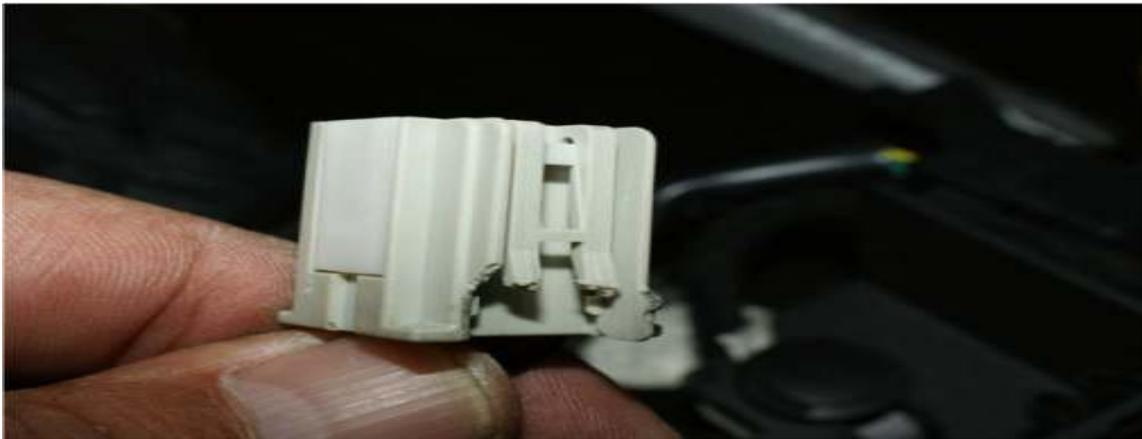
Lastly is the 12Volt power supply inside of console (Cigarette lighter in console). It's the same as the cigarette lighter plug . Remove the blue retaining clip and squeeze with your thumb to release it.
