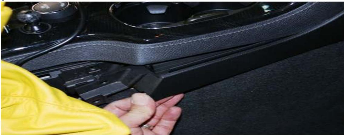
Once the “Ham-Bone” is out of the grooves pull down on it and it'll pop out (held in with clips by glove box)
