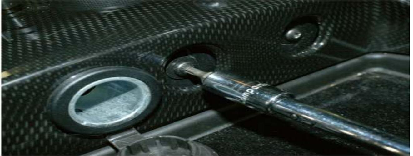
Your E-Brake boot hides (2) 7MM bolts behind it. Pull your E-Brake handle up... Then pull up on the E-Brake boot to reveal these 2 bolts
